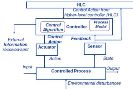
FIGURE 2 - GENERIC STRUCTURAL DIAGRAM OF CPS (ADAPTED FROM [1]).
